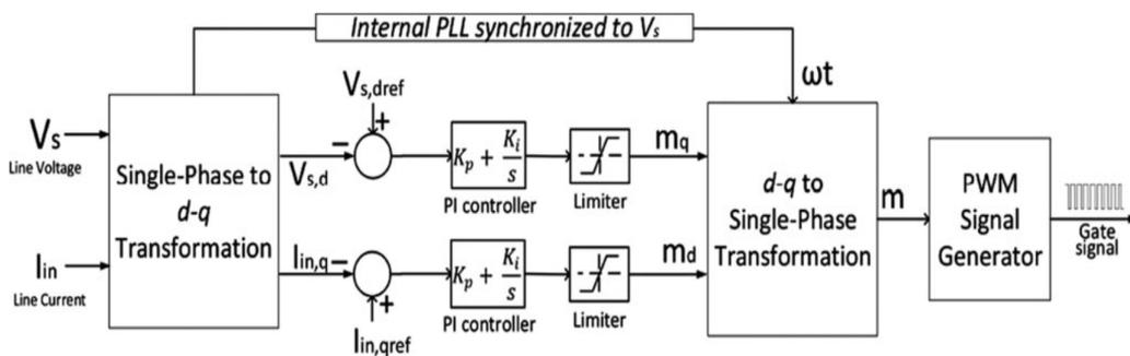
Fig.5. Improved control circuit for PFC and voltage support using ES.
