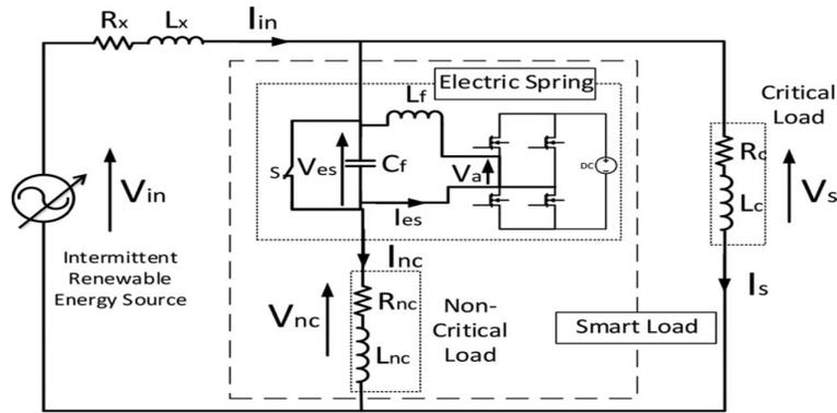
Fig. 1. ES in a circuit
