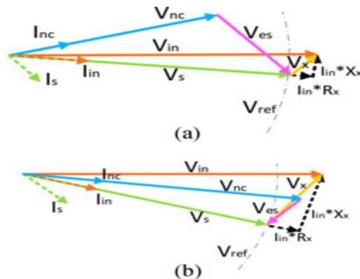
Fig. 2. Phasor diagrams of voltage and current for PFC and voltage support in (a) under voltage conditions and (b) overvoltage conditions.
