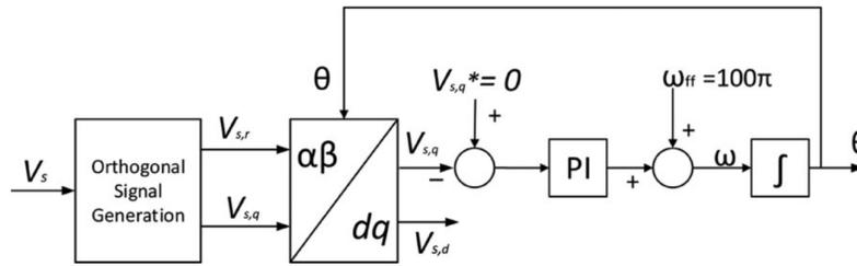
Fig. 4. Internal PLL using *d-q* transformation properties.
