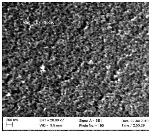
Fig. 2. Scanning electron microscope images of  $\text{TiO}_2$  layer the sample was annealed at  $500^\circ\text{C}$  for 30mins.
