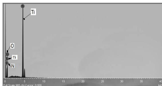
Fig. 3. X-ray microanalysis of the  $\text{TiO}_2$  layer showing the presence of Ti, O and N.
