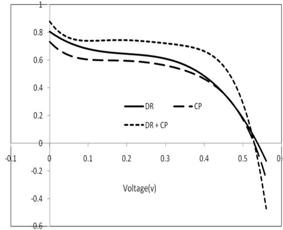
Figure 4: I-V- characteristics of the different cells at AM 1.5 illuminations.
