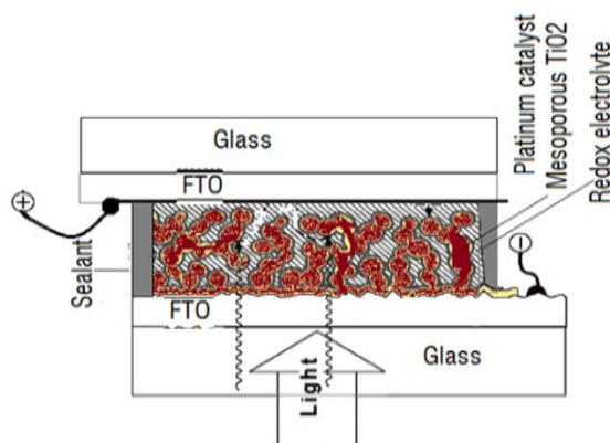
Figure 1. Schematic of a dye-sensitized photovoltaic cell.
