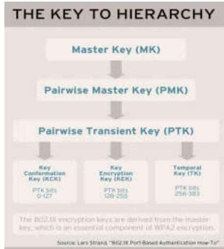
The Group Key Handshake is only used to disassociate a host or renew the GTK and uses the KEK generated during the 4-Way Handshake to encrypt the GTK.
