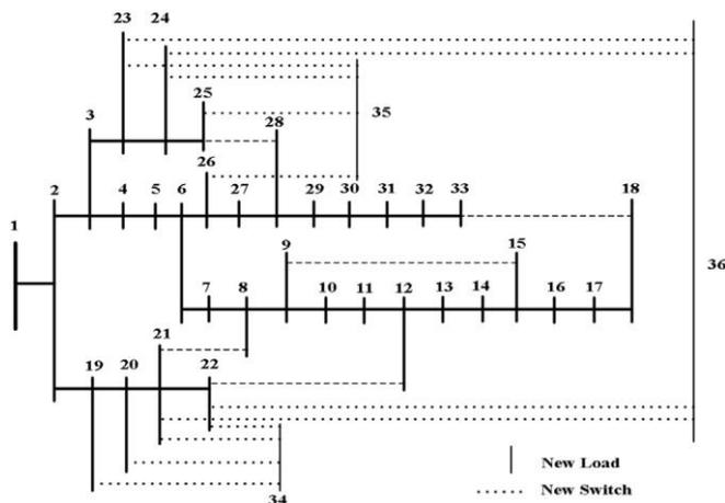
Fig.3. IEEE 33 bus distribution system with new load points
