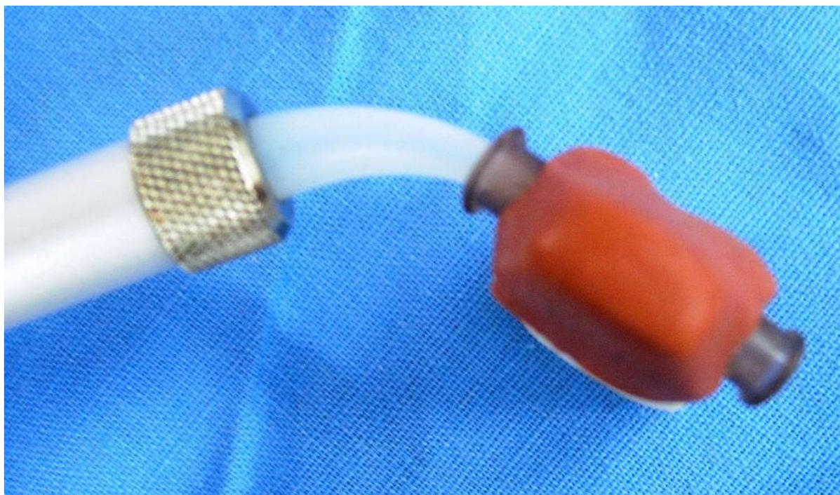
Figure 2: Light bodied polyvinylsiloxane injected through the inlet channel
