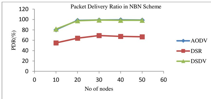
**Fig.1: Number of Nodes vs Packet Delivery Ratio**
