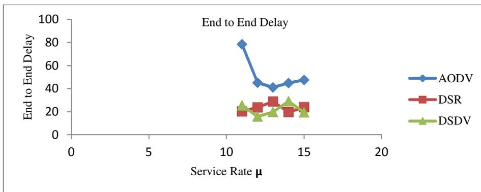
**Fig. 11: End to End Delay vs Service rate**
