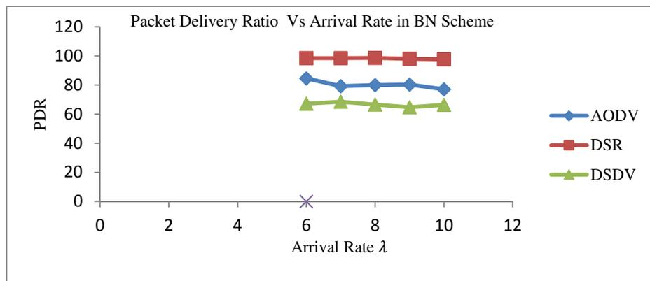
Fig. 7: Packet Delivery Ratio vs Arrival rate
