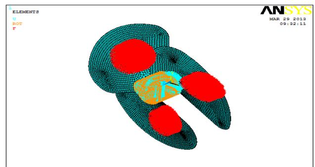
Figure 4.5: Thrust force applied on the blade
