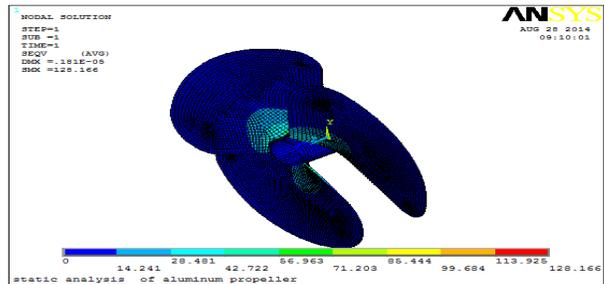
Figure 4.12: Von Mises stresses of aluminum propeller
