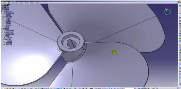
Figure 3.7: Final model after making groove for hole
