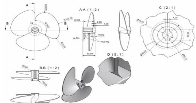
Figure3.1: Design parameters of propeller
