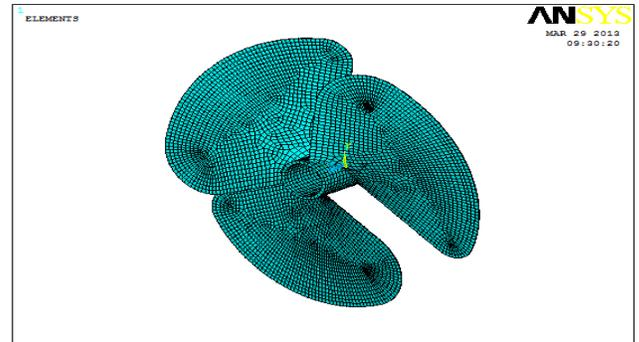
Figure 4.1: Meshed model in ansys of aluminum propeller
