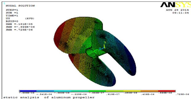
Figure 4.7: Deflection of aluminum propeller in Y direction
