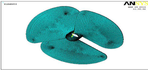
Figure 5.3: Meshed model of composite propeller
