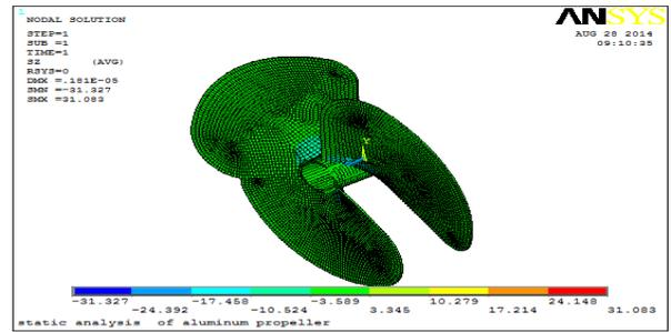
Figure4.11: Normal stress of aluminum propeller in Z direction
