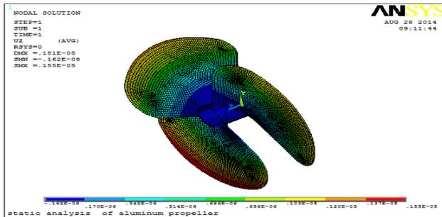
Figure 4.8: Deflection of aluminum propeller in Z direction
