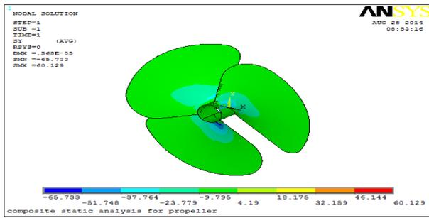
Figure5.11: Normal stress in composite propeller in Y direction
