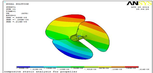
Figure 5.7: Deflection of a composite propeller with 8 layers in X direction
