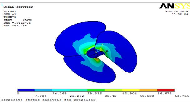
Figure5.13: Von mises stress of a composite propeller
