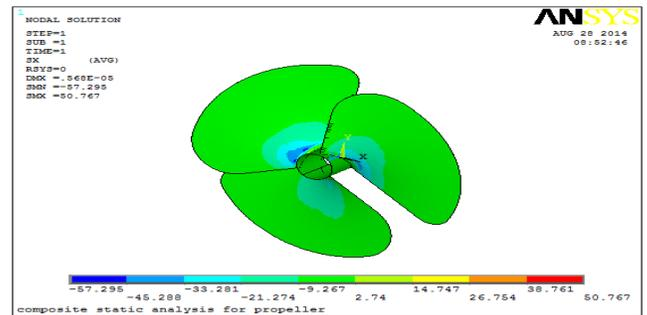
Figure 5.10: Normal stress in composite propeller in X direction
