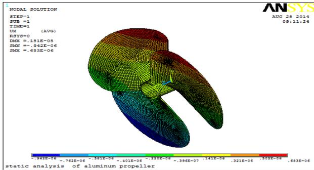
Figure 4.6: Deflection of aluminum propeller in X direction
