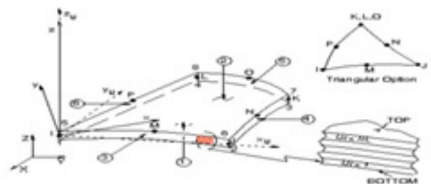
Figure: 5.2: SHELL 99 Linear layered structural shell.
