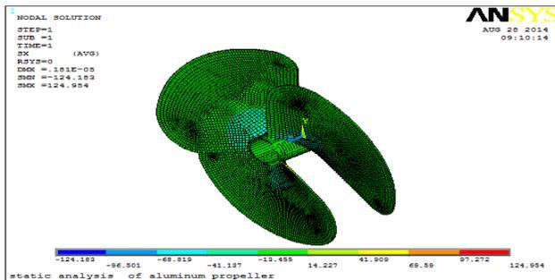
Figure 4.9: Normal stress of aluminum propeller in X direction
