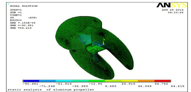
Figure 4.10: Normal stress of aluminum propeller in Y direction
