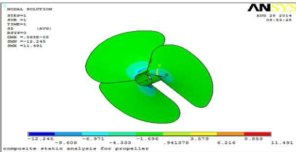
Figure5.12: Normal stress in composite propeller in Z direction
