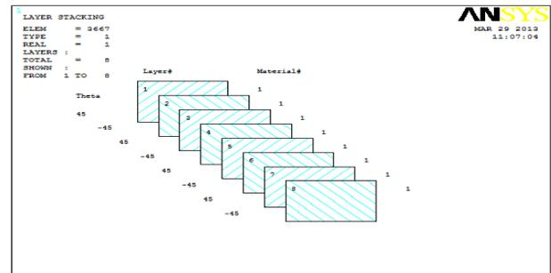
Figure5.1: Composite material layer stacking
