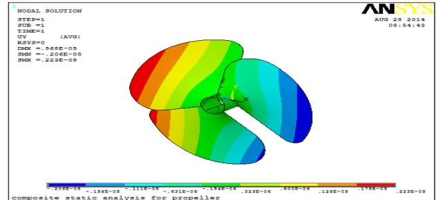
Figure 5.8: Deflection of a composite propeller with 8 layers in Y direction
