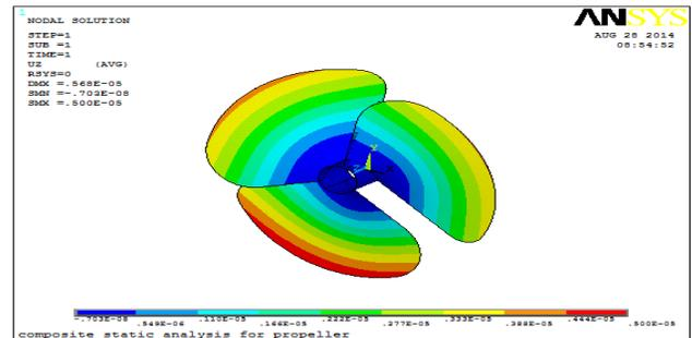
Figure 5.9: Deflection of a composite propeller with 8 layers in Z direction
