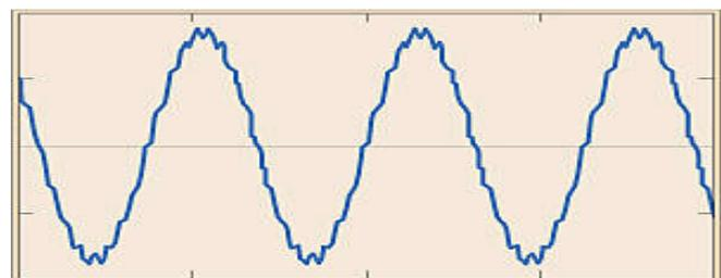
Fig.2.2 Fundamental waveform with 3<sup>rd</sup> harmonic content
