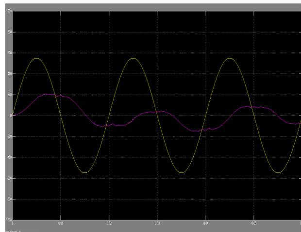
Fig.12.3.2 Waveform for voltage and current with SVC
