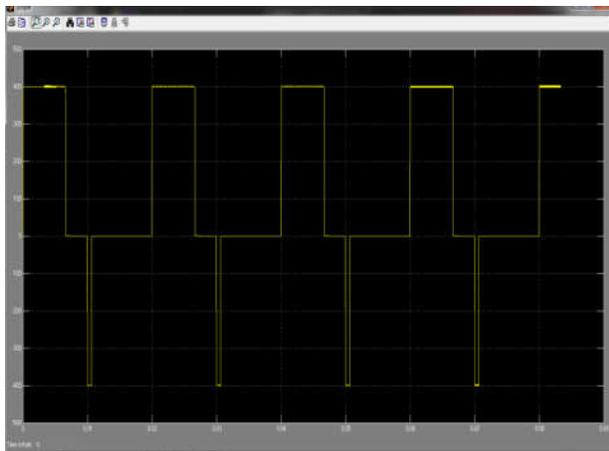
Fig.11.3 Line voltage of inverter without harmonic elimination
