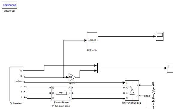
**Fig.12.1 Simulation of power system**
