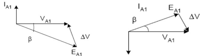
Fig.7.2 Phasor diagrams for leading and lagging mode
