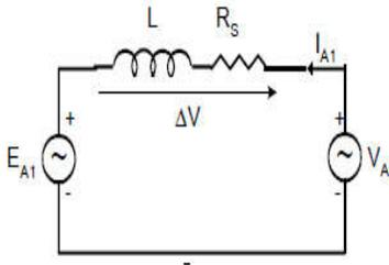
Fig.7.1 Per phase equivalent diagram of svc
