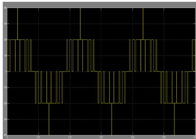
Fig.11.4 Line voltage for a three level inverter
