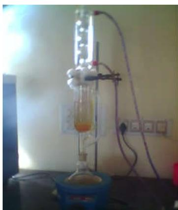
Fig :1 Soxhlet extraction
