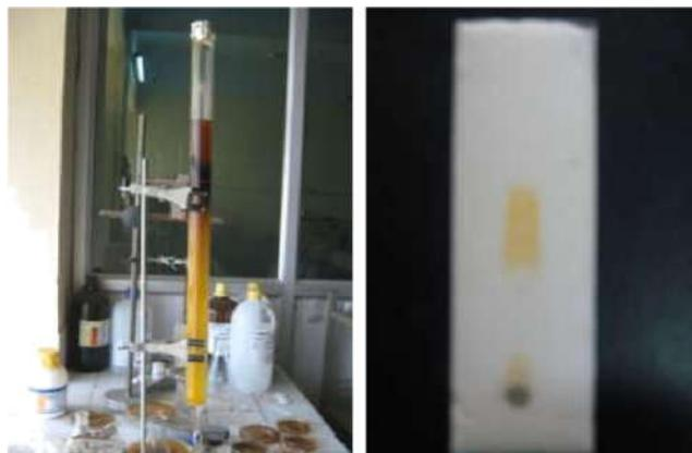
**Figure 6: Separation of Phenols from *A.L* by Column chromatography**
