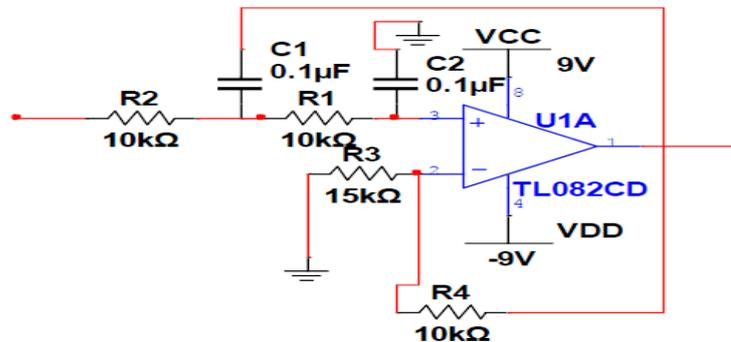
Figure: Schematic representation of low pass filter
