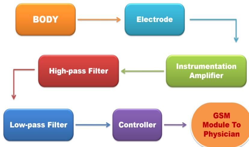
Figure: Block Diagram of Proposed System
