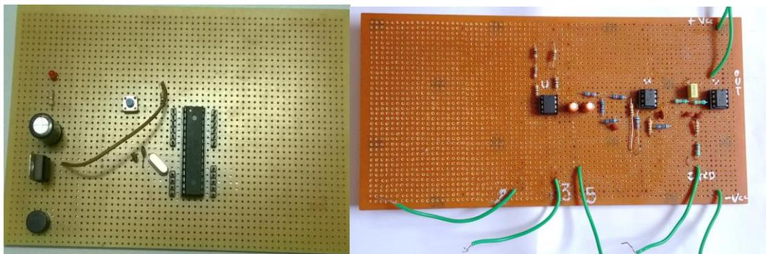
Figure: AVR microcontroller basic circuit and High pass, Low pass & Notch filter Circuit
