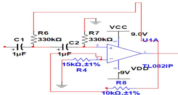
Figure: Schematic Representation of High pass filter
