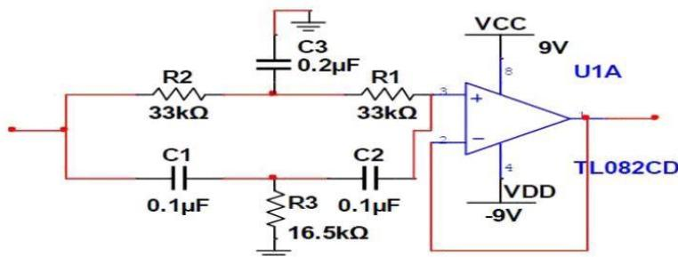
Figure: Schematic representation of Notch filter
