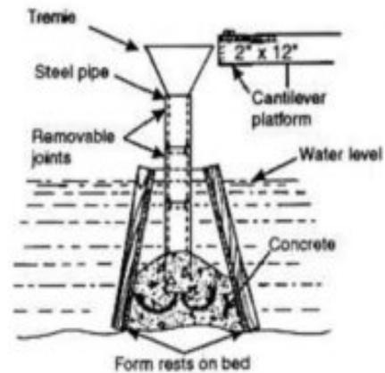
The principle of this method is that concrete is poured down a pipe or tube from above the surface and is forced into the mass of concrete already in place by the weight of concrete in the tube. The tube is surmounted by a hopper and the whole is suspended from a staging or frame, mounted so that it can be moved vertically when held by a crane. As the pour rises, sections of the tube can be removed to facilitate working. A convenient diameter for the tube is 8 to 16 times the maximum
