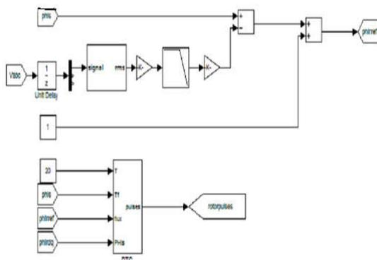
Figure: DTC block with rotor flux reference
