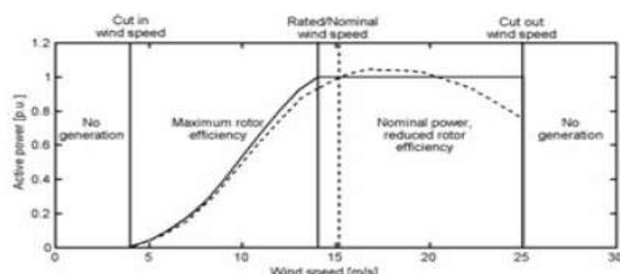
Fig.no.1.3.2. Typical power curve of a constant speed stall (dotted) and a variable speed pitch (solid) controlled wind turbine.
