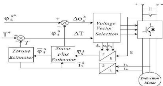
There are two hysteresis control loops, one for the Torque control and the other for the Flux control.
