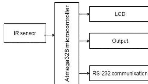
Fig. 3.3 Block diagram of Water dispensing system
