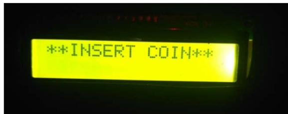
Then the Rs. 2 or Rs. 5 coin is inserted the LCD shows “Don’t waste water & Filling time” of water in seconds. The next step of the system is giving instruction as don’t waste water and display filling time is 15 seconds required for Rs. 2 coin and display filling time is 24 seconds required for Rs. 5 coin
