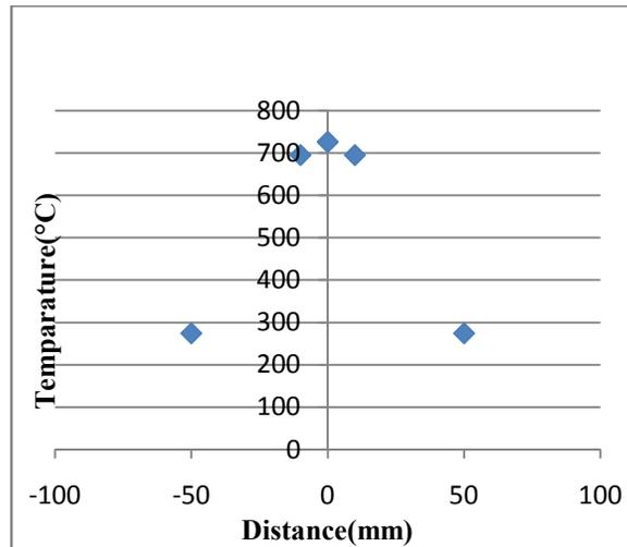
Fig 5.34 Temperature acting on the centre line of the specimen
