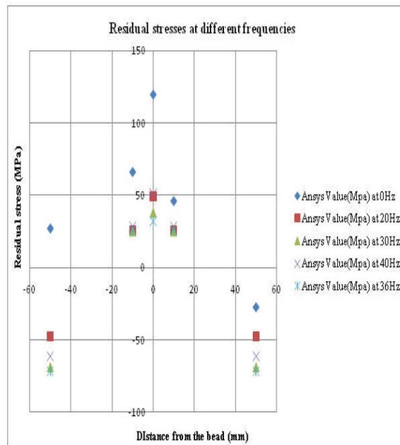
Fig 5.36 Residual stresses at different frequencies
