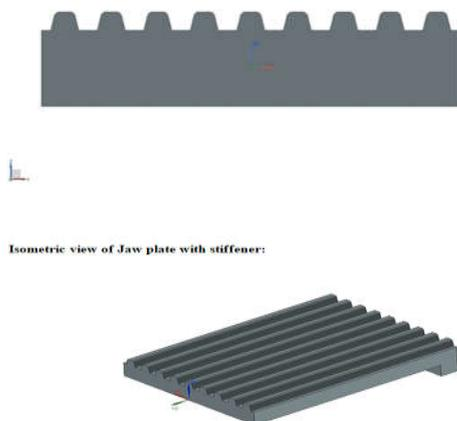
Figure 5 Shows the Isometric view of Jaw plate with stiffener
