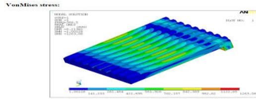
Figure shows the VonMises stress of Swinging jaw plate with stiffener
