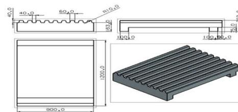
Figure shows the drafting of jaw plate with two stiffeners
