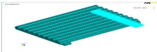
Figure shows Applied Boundary conditions on Swinging jaw plate with two stiffeners.
