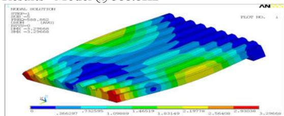
Figure Shows Mode shape 5@ 588.8Hz for Swinging jaw plate with stiffener
