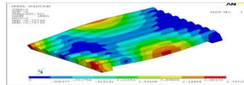
Figure 1 Shows Mode shape 5@ 585.3Hz for Swinging jaw plate with two stiffeners From the modal analysis,
