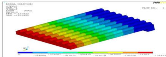
Figure Shows the Displacement vector sum of Swinging jaw plate with stiffener
