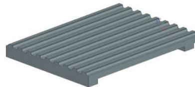
Figure Shows the Isometric view of Jaw plate with two stiffeners.
