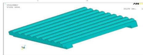
Figure shows the geometric model of the Swinging jaw plate with two stiffeners
