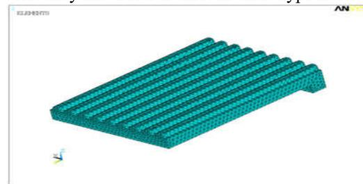
Fig: shows the meshed model of Swinging jaw plate with stiffener
