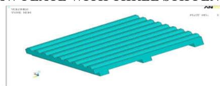
Figure shows the geometric model of the Swinging jaw plate with three stiffeners
