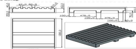
Figure shows the drafting of jaw plate with three stiffeners Isometric view of Jaw plate with three stiffeners:
