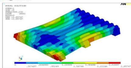
Figure Shows Mode shape 5@ 568.2Hz for Swinging jaw plate with three stiffeners
