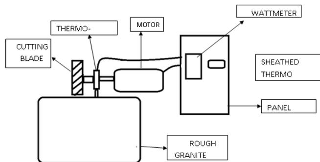
Figure 1: Showing line diagram of experimental setup
