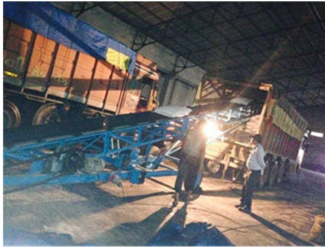
Fig. 7. Snapshot of transferring fertilizer bag through stacker machine
